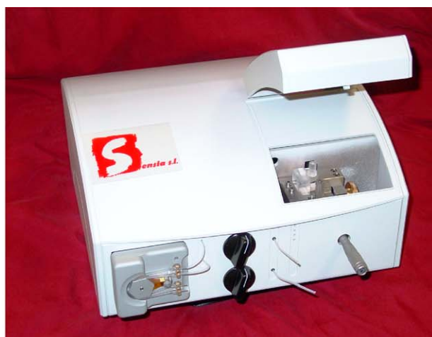
Fig. 1. Portable SPR sensor prototype system including sensor, optics, electronics and flow delivery system: (a) scheme of the SPR device and (b) commercial \beta -SPR platform.
